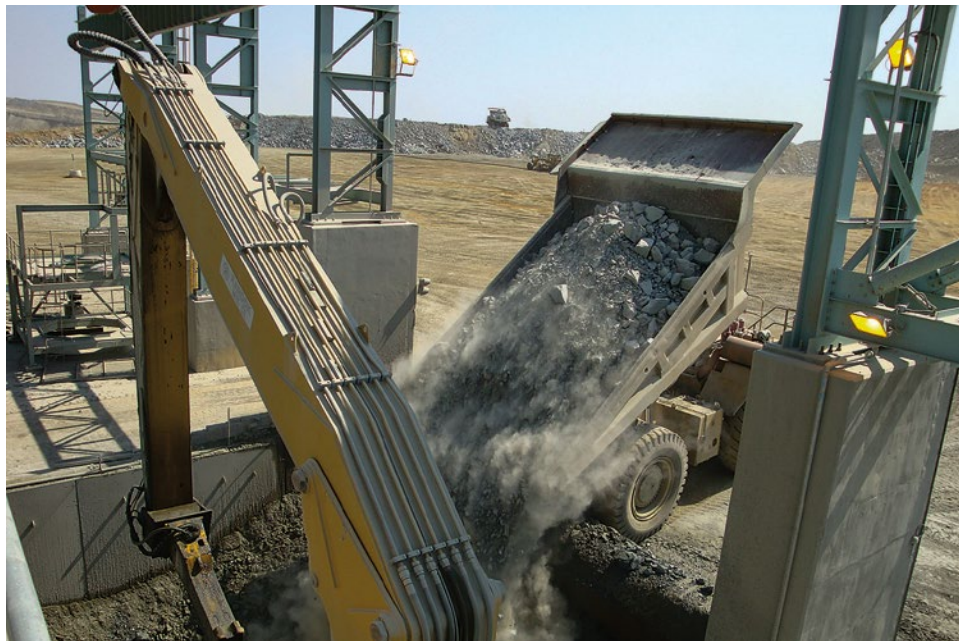
Komatsu HD785 truck dumping ore into crusher at Phoenix Nickel
